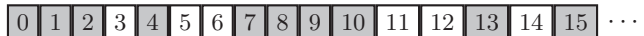
Fig. 2. An Example of Channel II: In any sliding window of length W = 5 there is either a single erasure burst of length up to B = 3 and possibly one isolated erasure, or N = 2 isolated erasures.
