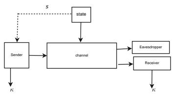
Fig. 1. Wiretap channel controlled by a state parameter. The channel transition probability  $p_{y_r,y_e|x,s}$  is controlled by a state parameter s. The entire source sequence  $s^n$  is known to the sender but not to the receiver or the eavesdropper. The sender and receiver generate a secret key  $\kappa$  at the end of the transmission.
