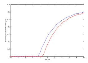
Fig. 4. Optimal fraction of power that must be allocated to the state  $\mathbf{s}_r = 0$  to maximize the secret-key rate with Gaussian inputs. The curve marked with a  $(\times)$  denotes the case of public discussion while the other curve denotes the case of no public discussion.
