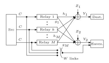
Figure 1. The wiretapped diamond-relay channel.
