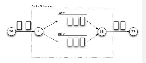
In essence, a PacketScheduler object receives packets from one or more traffic generators (TG), and forwards packet to a single traffic sink (TS).
