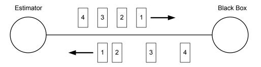
Your task is to build a software tool, called the "Estimator". The Estimator is a Java program which sends sequences of probe packets to the Black Box. The probe packets are returned by the Black Box to the Estimator. The Estimator creates timestamps for each packet sent to the Black Box and for each packet returning from the Black Box. Using these timestamps, the Estimator computes the parameters of the Black Box.
