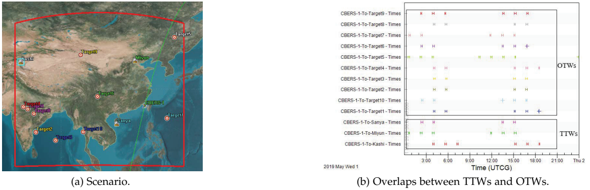
Fig. 2. Illustration of overlaps between TTWs and OTWs, for one observation satellite, three GSs, and ten targets. (a) The simulation scenario. (b) The TTWs and OTWs obtained via the satellite tool kit. It can be seen that the TTWs and OTWs frequently overlap.
