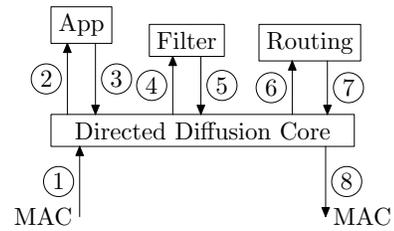
Fig. 2. Directed Diffusion Network Stack
