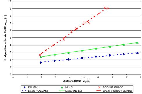
Fig. 3. Showing effect on performance when the inter-vehicle distance estimation error is varied
