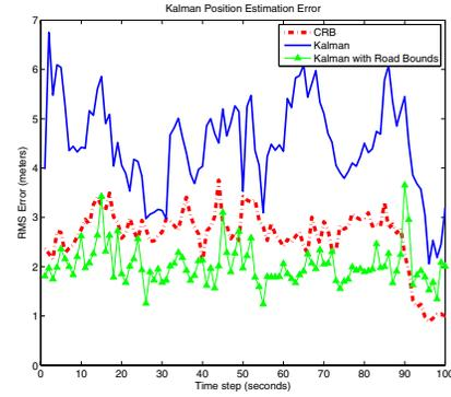
Fig. 1. Cramér-Rao bound for position estimates versus our Kalman filter based solution, lower curve shows performance gain by forcing the position estimate to be within the confines of the road
