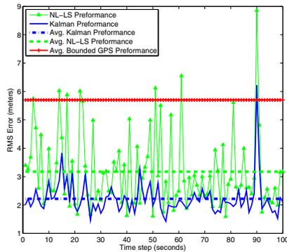
Fig. 4. Comparison of Nonlinear Least of Squares approach to our Kalman filter based approach, also the performance of using GPS with a mapping module is shown for reference
