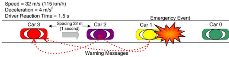
Fig. 1. Model for chain of car collisions.
