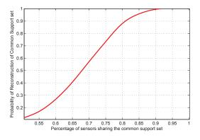
Fig. 3. Reconstruction of the common support set in an imperfect G-JSM model for J = 100, N = 50, M = 25,  $K_C = 3$  and  $K_j = 3$ .
