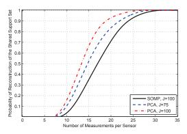
Fig. 1. Reconstruction of the common support set in G-JSM using PCA and SOMP for  $J \in \{75, 100\}, N = 50, K_C = 5$  and  $K_j = 5$ .
