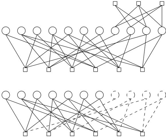
Fig. 3. Two concatenated LDPC codes. Top: New parity checks succeed with crossover probability  $p_2$ . Bottom: When the new checks are decoded, enough symbols are revealed in the original code to permit decoding.
