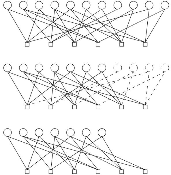
Fig. 2. LDPC codes in a revealing source. Top: The full code, when  $b = 1$ . Middle:  $b < 1$ , and the last four symbols are revealed. Bottom: The code when the last four symbols are removed, which can be used for inversion probability  $p$ .
