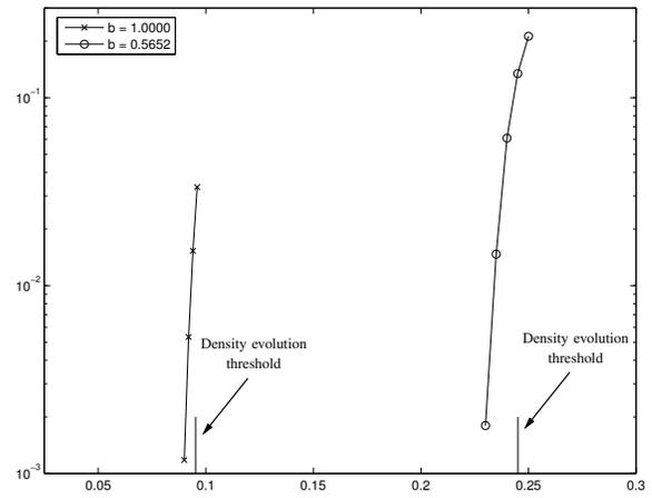
Fig. 4. Experimental results for the given code, for sources  $(1, 0.0953)$  and  $(0.5652, 0.2451)$ .
