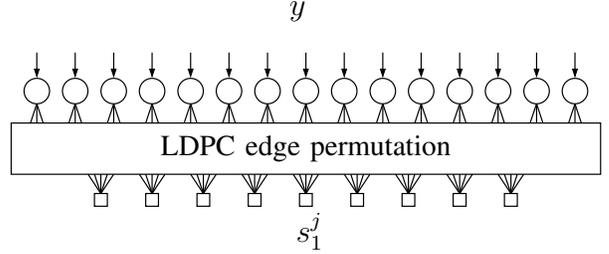
Fig. 1. LDPC-based Slepian-Wolf decoders at a corner point (top), and a non-corner point (bottom).
