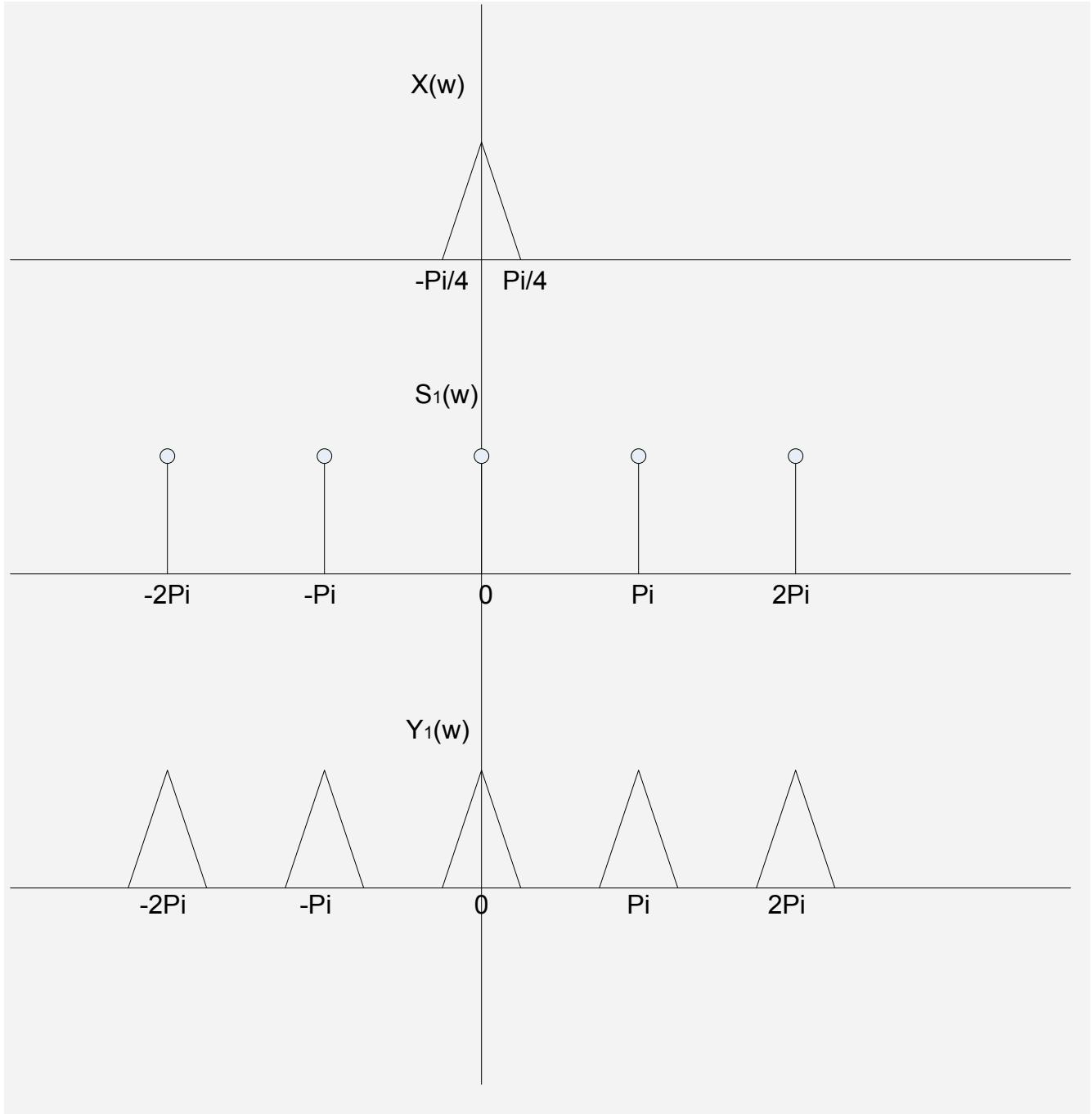
(a) We have  $y_1(n) = \begin{cases} x(n) & \text{if } n \text{ even} \\ 0 & \text{otherwise} \end{cases}$  which we can rewrite considering (b) and (c) as:
