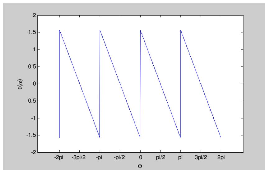
(I) The Fourier transform of the signal  $y(n) = x(n - 4)$  is  $Y(\omega) = \exp(-j4\omega) \cdot X(\omega)$  and the corresponding filter is  $H(\omega) = \frac{Y(\omega)}{X(\omega)} = \exp(-j4\omega)$
