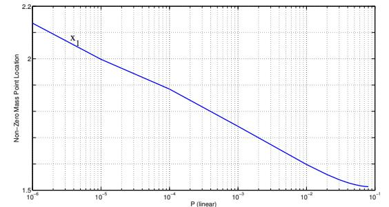
Fig. 5. The non zero mass point location versus the SNR value  $P$  at very low SNR region .
