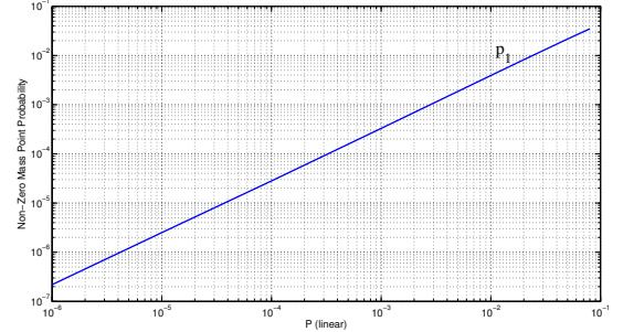
Fig. 4. The non zero mass point probability versus the SNR value  $P$  at very low SNR region.
