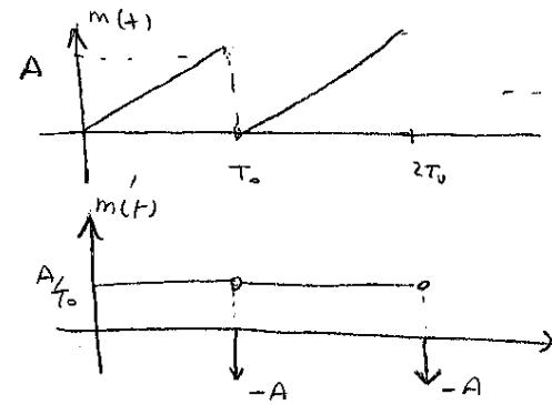
Therefore,  $s_{pm}(t)$  is a cosine with a frequency  $f_c + \frac{K_p}{2\pi} \frac{A}{T_0}$  when at  $nT_0$  will have phase shifts of  $-K_p A$
