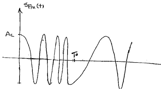
i.e., signal is a cosine with an instantaneous frequency increasing from  $f_c$  to  $k_f A$  and then resetting to  $f_c$  at  $nT_0$ .
