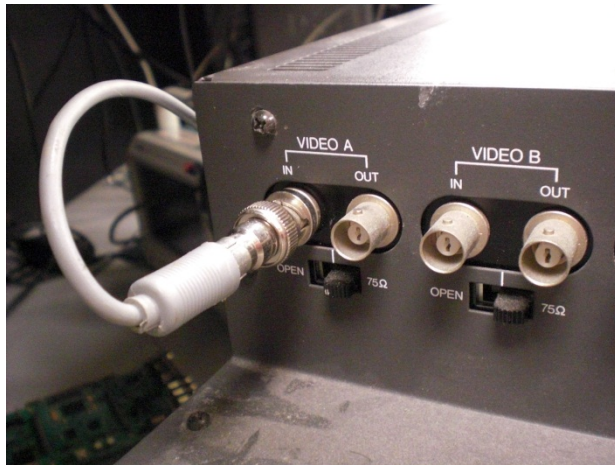
Fig. 15. Connection of Video Output and TV.
