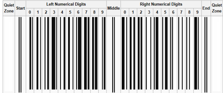
Fig. 2. Number Encoding (“Universal Product Code.”)
