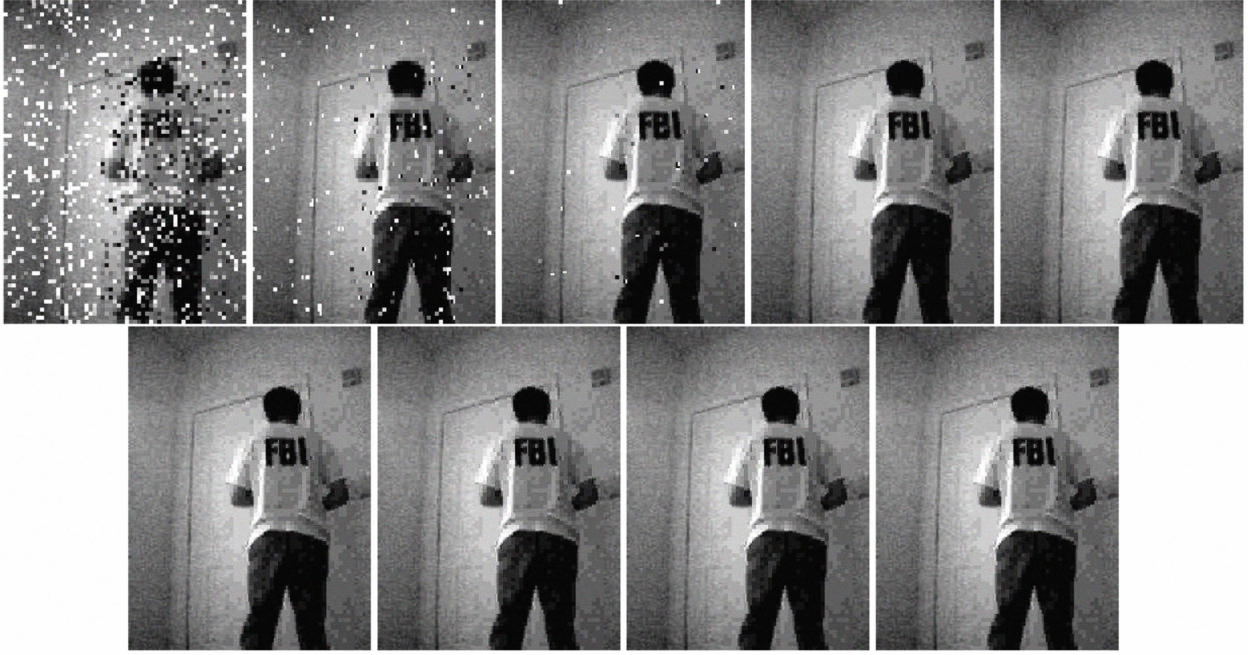
Fig. 4. Examples of S/DISCUS decoded images. In these cases, S/DISCUS encodes the quantized 4 \times 4 integer DCT coefficients of the images (with an equivalent H.264 Quantization Parameter of 20). The number of coded coefficients of each block ranges from 1 to 9, where the corresponding images are sequentially ordered from top-left to bottom-right. The quantized coefficients of different frequencies are mixed and encoded together.
