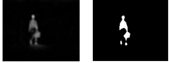
Figure 4. Filtered image on the left and mask after threshold on the right.
