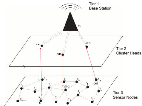
Fig. 2. Hierarchical network structure for the FSOSN based on node function specialization.
