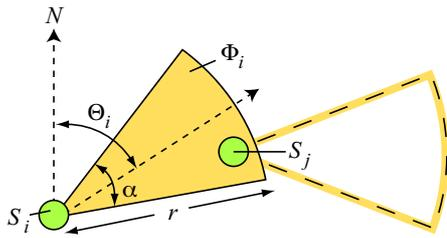
Fig. 1. Node  $S_j$  can only hear node  $S_i$  if it falls into  $S_i$ 's communication section.
