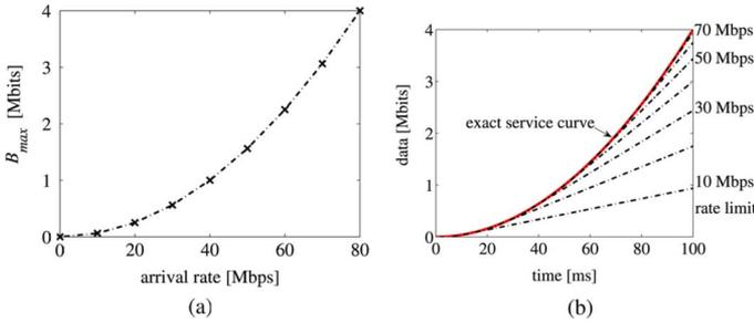
Fig. 4. Service curve estimation with rate scanning. (a) Maximum backlog  $B_{\max}(r)$ . (b) Rate scanning results with different rate limits.
