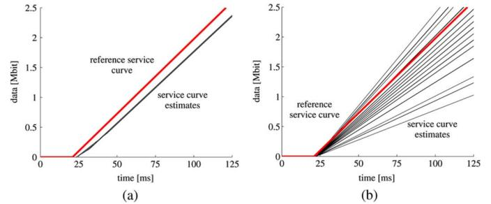
Fig. 8. Experiment 1: Service curve estimates with CBR cross traffic (Each of the graphs shows the reference service curve and the results of 100 repeated estimates of the service curve). (a) Rate Scanning. (b) Rate Chirp.
