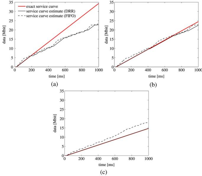
Fig. 3. Example: Passive measurement simulation with a video source. (a)  $C = 70$  Mbps. (b)  $C = 50$  Mbps. (c)  $C = 30$  Mbps.
