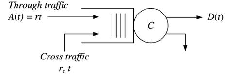
Fig. 6. FIFO system with probe and cross traffic.
