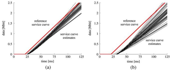
Fig. 9. Experiment 2: Rate scanning with different cross traffic. (a) Exponential cross traffic. (b) Pareto cross traffic.
