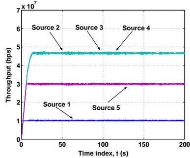
**Fig. 7. Experiment 3** - Throughput achieved by multipath-AIMD with PPF correction ( $K = .00001$  Mbps).
