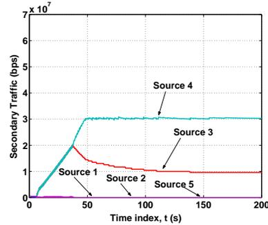
**Fig. 10. Experiment 4** - Secondary traffic achieved by multipath-AIMD with PPF correction ( $K = .01$  Mbps).
