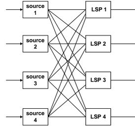
**Fig. 2.** The simplified network model. LSP  $i$  is the primary path for source  $i$ .
