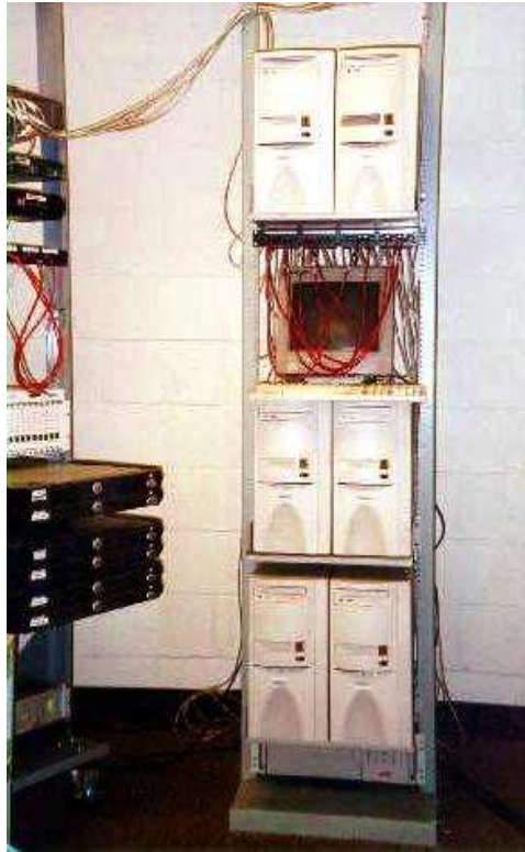
Figure 6.1: The testbed used for the experiments. Our testbed consists of 6 PC-routers and Fast Ethernet hardware.
