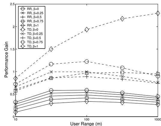
Fig. 5. Effect of user range and proportion of downlink data, for  $\frac{P_{ar}}{N} = 40$ ,  $\frac{P_m}{N} = 20$ ,  $\alpha = 2$ , and  $n = 16$ .
