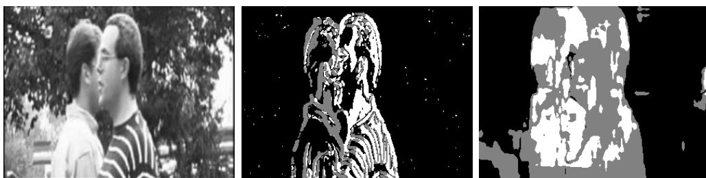
Figure 4: (left) source image. (middle) motion segmentation result achieved by our fully-enabled motion estimation and segmentation algorithm. (right) result achieved by local flow computation followed by MOG clustering.
