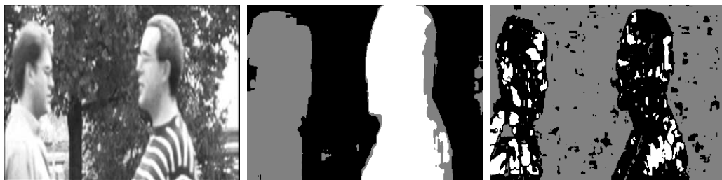
Figure 1: Local flow computation followed by clustering is an ineffective, unreliable way to obtain motion field and segmentation estimates. At left, the first of an input source image pair. At middle, the result obtained by applying the local optical flow estimation method [6] with an aperture of \pm 15 . At right, the result obtained by applying the local optical flow estimation method [6] with an aperture of \pm 5 . In both cases the smoothing parameter \sigma = 2.75 . Note that an aperture of \pm 15 was the smallest value that yielded reasonable segmentation results in our experiments. Clearly in this (the optimal) case, the achieved segmentation is of very low spatial resolution, with large regions of segmentation error.
