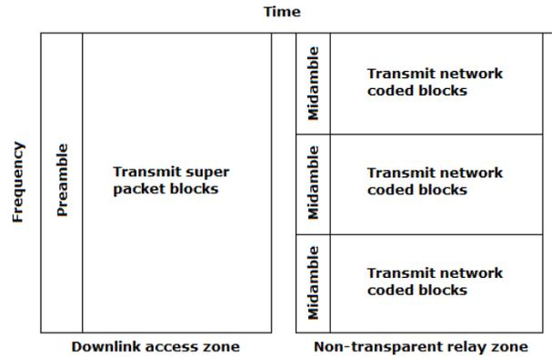
Fig. 2. Proposed downlink sub-frame structure.
