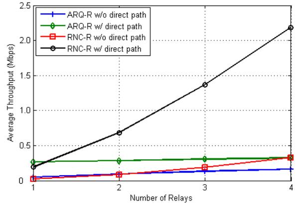
Fig. 4. Average throughput vs number of relays, with and without direct path
