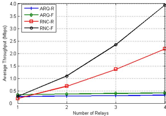
Fig. 6. Average throughput vs number of relays, floating and rigid acknowledgement
