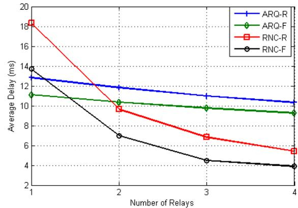
Fig. 7. Average delay performance vs number of relays, floating and rigid acknowledgement
