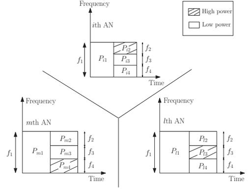
**Fig. 2.** Frame structure and power configuration of three ANs  $i$ ,  $l$ , and  $m$ .
