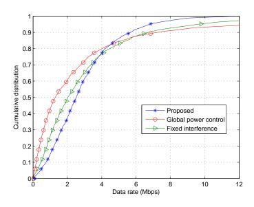
Fig. 2: Comparison of the proposed coordinated uplink user scheduling and power control method with two baseline methods in term of cummulative distribution function of user rates.
