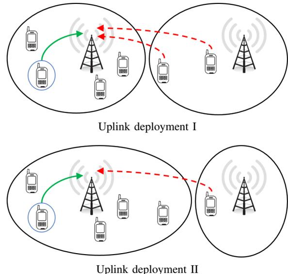
Fig. 1: The uplink interference pattern for the circled user is strongly affected by the cell association and scheduling rules of neighboring BSs. Here, the solid lines represent the desired signal while the dotted lines represent the interfering signal.
