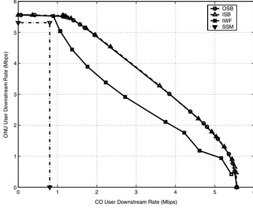
Fig. 2. Rate Region for Two Downstream ADSL Users
