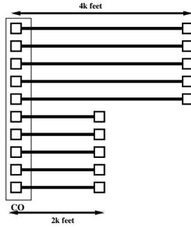
Fig. 6. Loop Topology for 10-User VDSL
