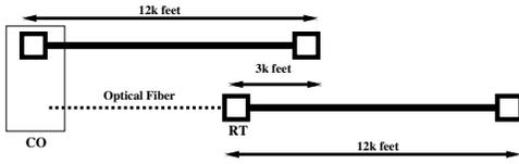
Fig. 1. Loop Topology for Two Downstream ADSL Users
