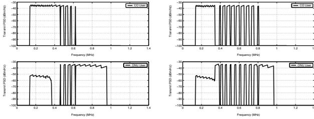
Fig. 3. OSB (left) and ISB (right) power spectral densities for two distributive ADSL users at equal rate. Power spectral densities for both CO-based (top) and RT-based (down) lines are plotted.
