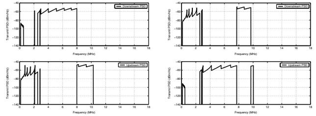
Fig. 5. Downstream (top) and upstream (bottom) power spectral densities for 5-user full duplex VDSL at equal rate. The power spectra depend on the ordering in iteration in ISB. Downstream-upstream order is on the left, and the upstream-downstream order is on the right.
