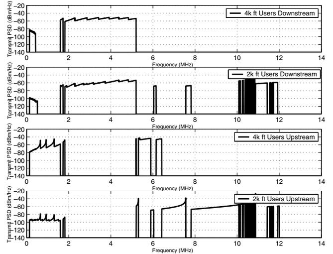
Fig. 7. Power spectral densities for 10-user full duplex VDSL at maximum minimal rate
