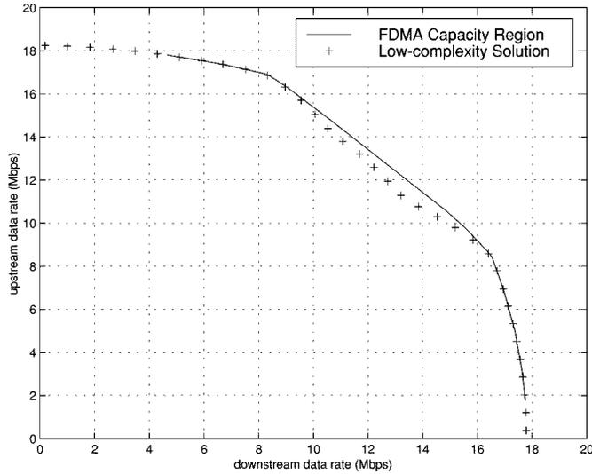
Fig. 7. The achievable rate region with frequency-division duplex in a 500-m VDSL line.
