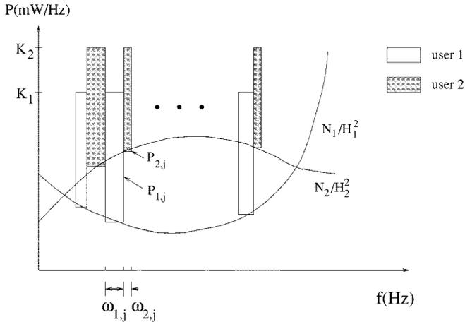
Fig. 3. Optimization with frequency-division multiple access.
