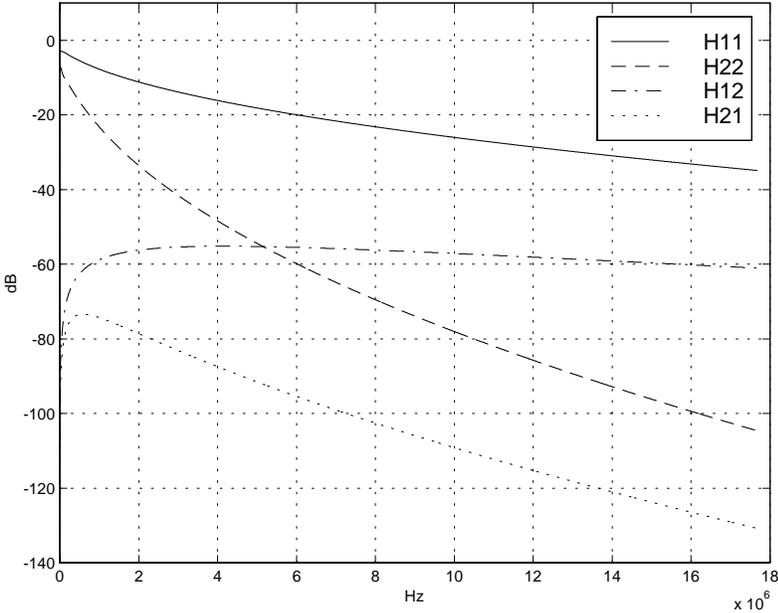
Figure 4.6: Channel and crosstalk transfer functions of 3000ft and 1000ft lines
