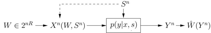
Figure 3.3: Channel with non-causal transmitter side information
