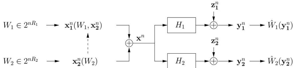
Figure 3.5: Coding for vector broadcast channel
