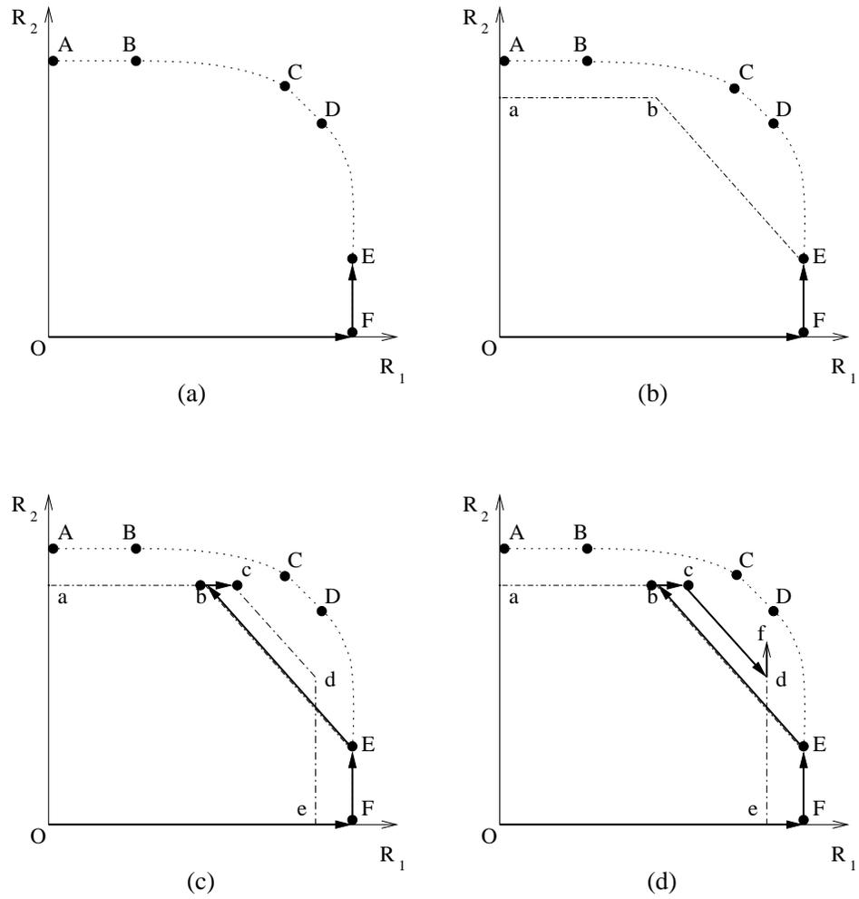
Figure 2.4: Illustration of iterative water-filling
