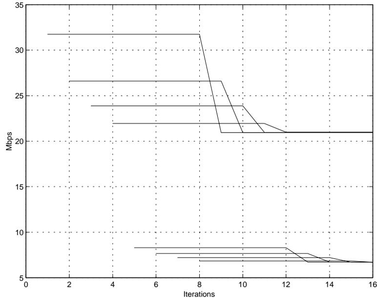
Figure 4.8: Convergence of iterative water-filling algorithm
