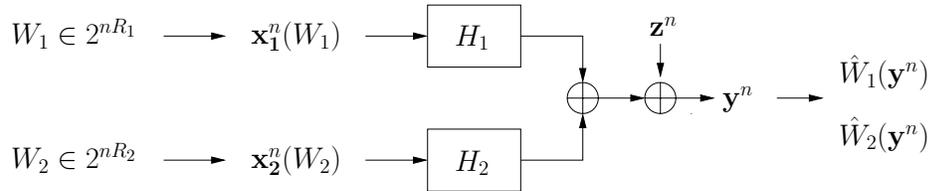
Figure 2.2: Gaussian vector multiple access channel
