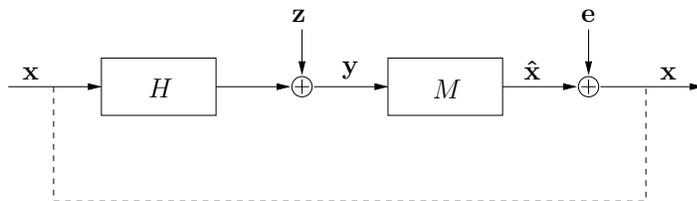
Figure 3.6: MMSE estimation in a Gaussian vector channel
