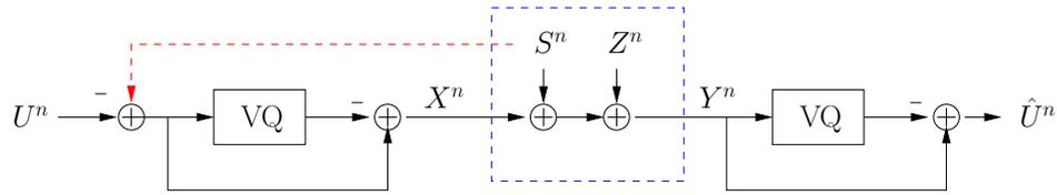
Figure 3.14: Precoding via vector quantization
