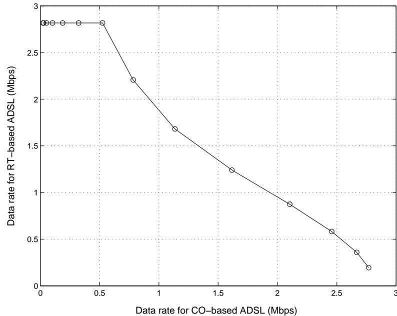
Figure 4.11: Competitively optimal downstream rate region of two ADSL lines
