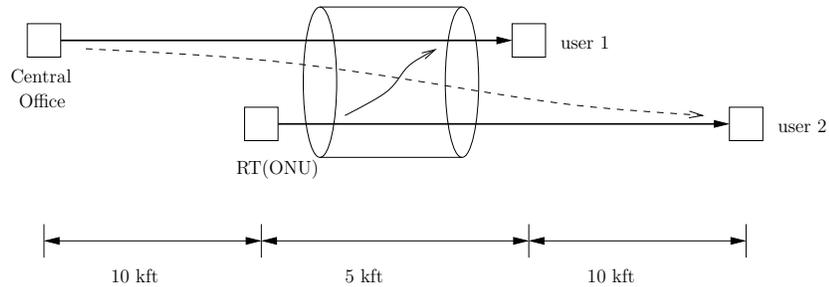
Figure 4.10: CO-based ADSL vs. RT-based ADSL
