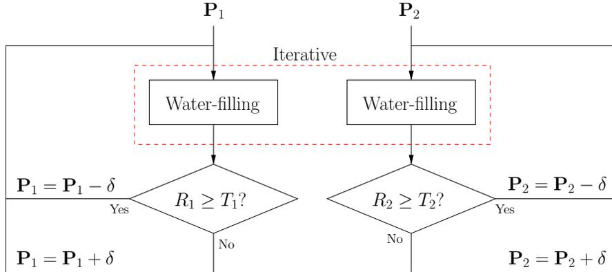
Figure 4.5: Distributed power control by iterative water-filling
