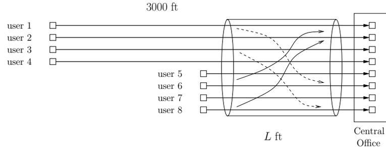
Figure 4.7: Loop topology for VDSL upstream power back-off
