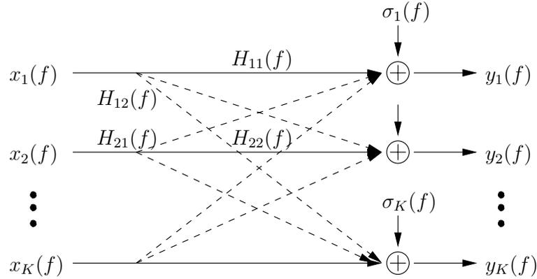
Figure 4.2: Gaussian interference channel model
