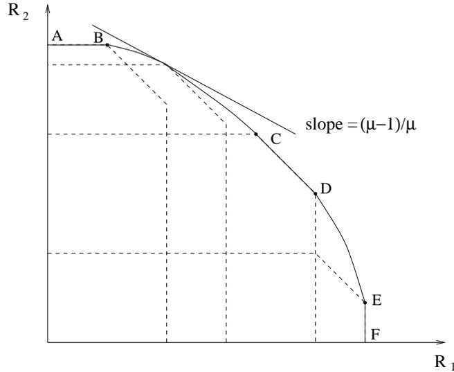
Figure 2.3: Capacity region of a Gaussian vector multiple access channel
