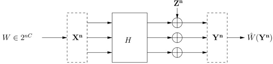
Figure 1.4: Gaussian vector channel
