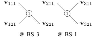
(b) Conditions for interference alignment in a (3, 2, 2, 5) network with one additional antenna at BS 2.
