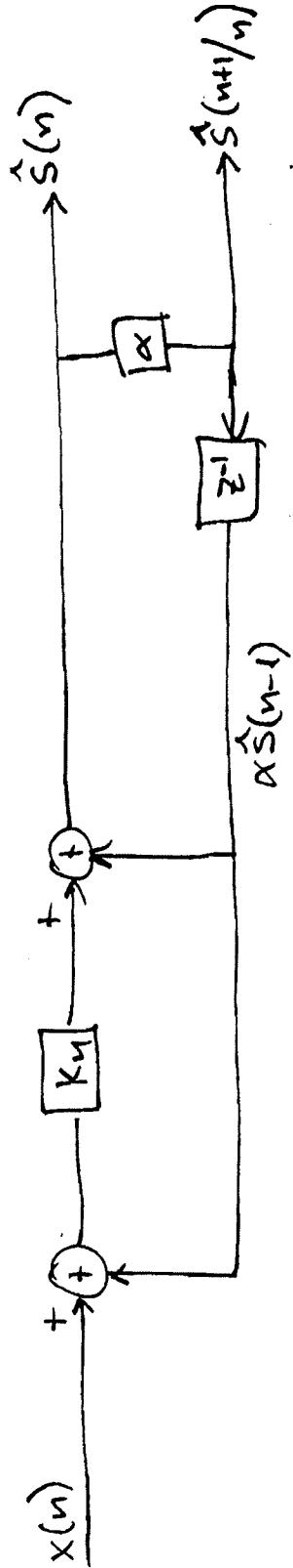
System to perform simultaneous filtering and prediction.
