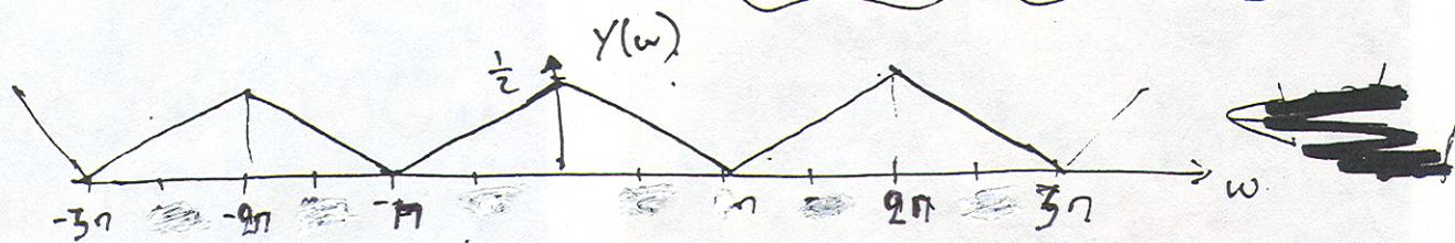
Aliasing occurs but  $x(n)$  can still be reconstructed from  $y(n)$  by upsampling by 2 and then bandpass filtering. Note however that we must know a priori that  $x(n)$  is high-pass to select the appropriate filter.
