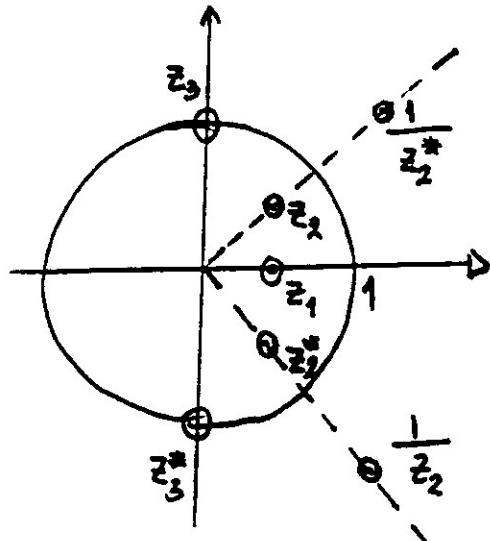
\* If a real linear phase FIR Filter has a zero at  $z=z_2$  then it also has zeros at  $z=\frac{1}{z_2}$ ,  $z_2^*$ ,  $\frac{1}{z_2^*}$
