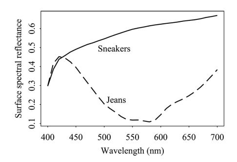
Figure shows the surface spectral reflectance from: (1) orange sneakers; and (2) faded blue jeans. The reflectance function is denoted  $S(\lambda)$
