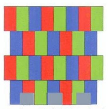
TRADEOFFS: Most flat-panel displays today, with their I:I:I ratio of red, green, and blue elements, compromise on power consumption and resolution. These elements, or subpixels, are arranged in either a conventional stripe pattern [left] or a delta pattern [right]. Because light from the blue subpixels does little to help the eye resolve images, most of it goes to waste.
