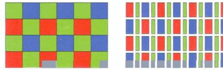
EASY ON THE EYES: The Bayer pattern [left] saves power by including extra subpixels in the color green, which the human visual system resolves with particular efficiency. The PenTile Matrix [right] yields even better results by changing the size and arrangement of the pixels.
