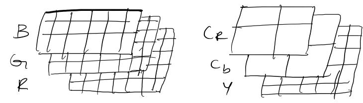
While R,G,B components are usually equally important (intensity wise) Y, C<sub>b</sub>, C<sub>r</sub> components are not. In this case Y is more important than C<sub>b</sub>, C<sub>r</sub>.
