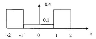
Use the Max-Lloyd algorithm to design a 1-bit non-uniform quantizer (see last page for useful formulas). Use a uniform quantizer to initialize the algorithm. Use at least one iteration of the algorithm and comment on the final decision boundaries and reconstruction values. (5 points)
