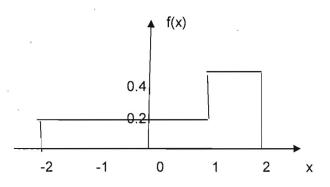
Use the Max-Lloyd algorithm to design a 2-bit non-uniform quantizer. Use the settings for a uniform quantizer to initialize the algorithm. What are the decision boundaries and reconstruction levels at the end of recursion (iteration) 1. What is the corresponding MSE distortion for this quantizer? (3 points)
