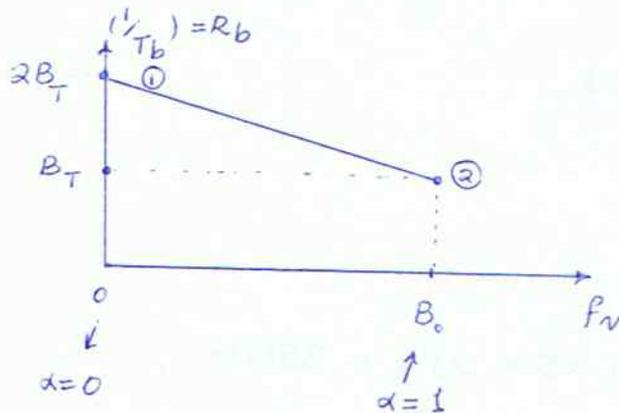
$$\Rightarrow \textcircled{1} \text{ at zero excess BW } \alpha = 0 \quad f_N = 0 \quad B_T = 3k \Rightarrow \underline{R_b = 6 \text{ kbps}}$$
