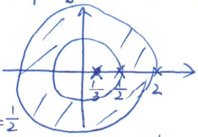
and the poles  $p_1 = \frac{1}{3}$ ,  $p_2 = \frac{1}{2}$  provide the causal parts,  $p_3 = 2$  provides the anti-causal part.
