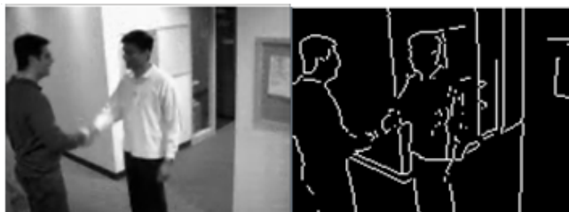
Figure 2: Edge detection using the Sobel algorithm
