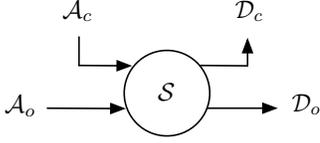
Fig. 3. Single fading channel with cross traffic.
