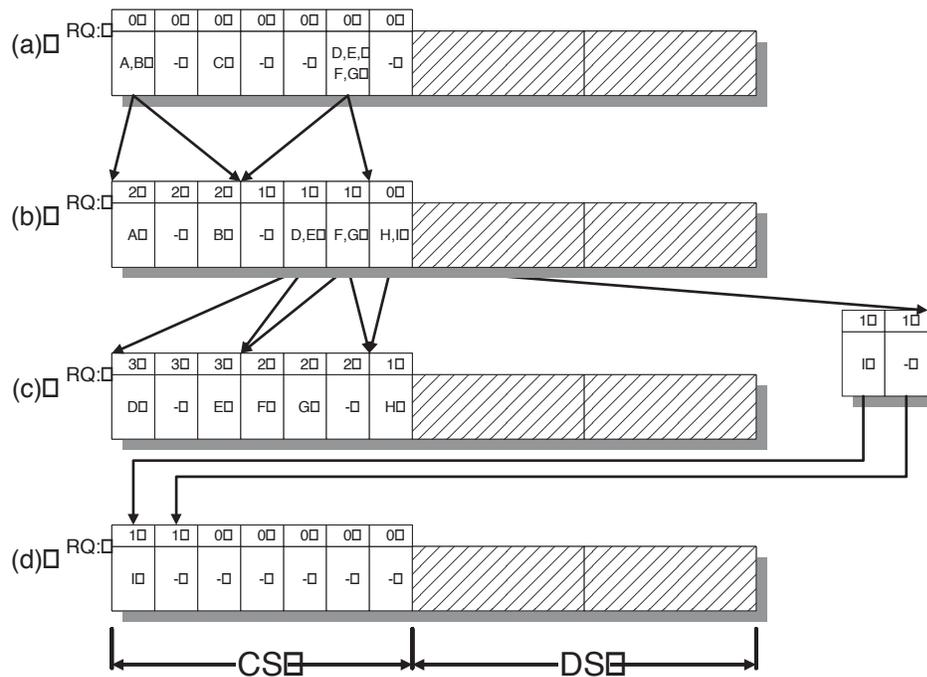
Figure 3.1: Collision Resolution Example
