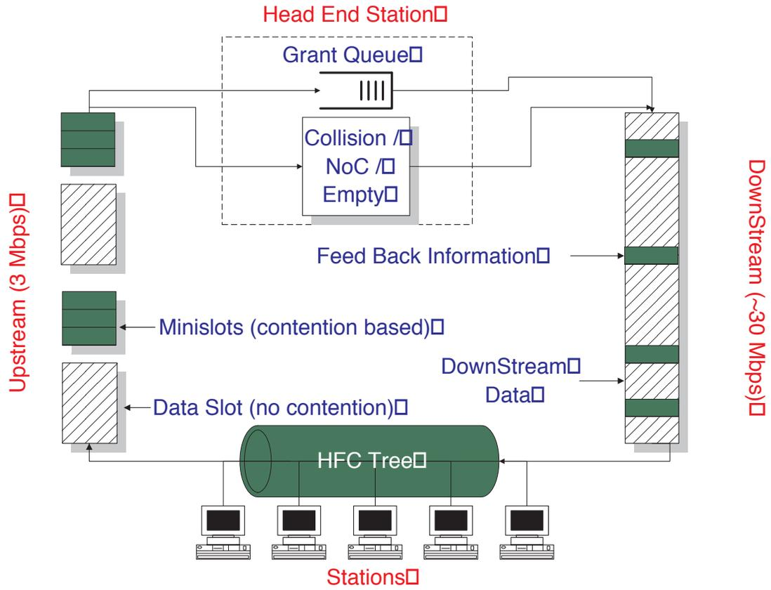
Figure 2.1: Media Access Control in HFC Networks.
