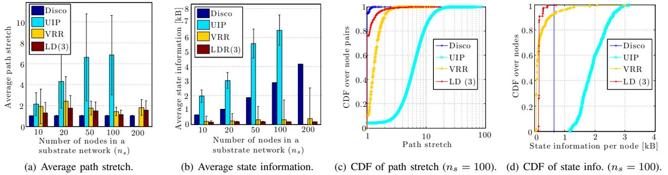
Fig. 8: Static multi-substrate network ( $\alpha = 2.2$ ,  $\beta = 2.2$ ,  $s = 25$ ).
