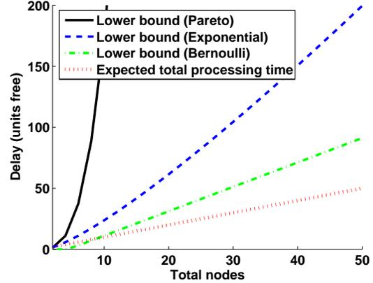
Fig. 4. Lower bounds for the median of the end-to-end delay for different packet size distributions as a function of the number of nodes. ( $z = .5$ ,  $C = 1$ ,  $\rho = 0.75$ , mean packet size 1, packet spacing  $1/\rho$ ).
