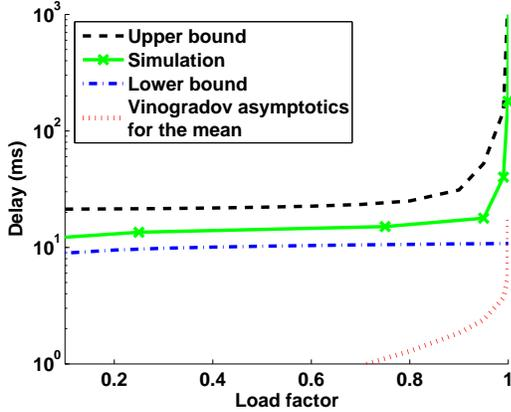
Fig. 3. End-to-end delay  $w_H(z)$  as a function of the load factor  $\rho$  (path length  $H = 25$  nodes,  $z = 1 - 10^{-6}$ ,  $C = 100$  Mbps,  $\mu^{-1} = 400$  Bytes.)
