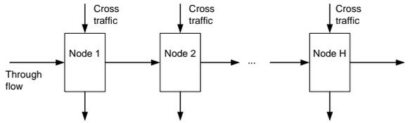
Fig. 1. A tandem network with cross traffic.
