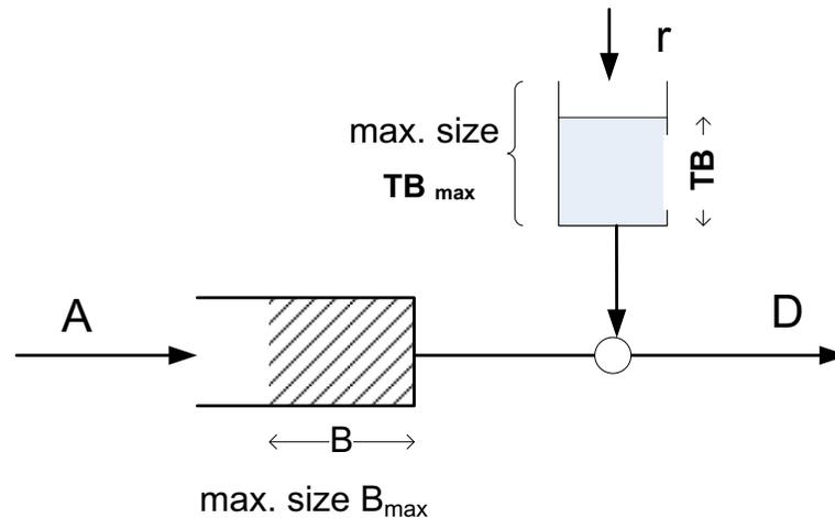
The token bucket for this Lab receives data from a traffic generator on a UDP port and transmits the output to a traffic sink, specified in terms of an IP address and a UDP port. This is illustrated below.
