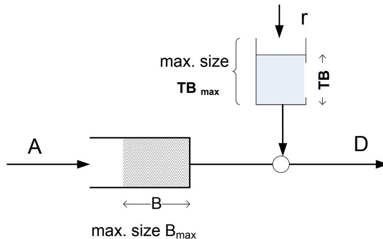
The token bucket for this Lab receives data from a traffic generator on a UDP port and transmits the output to a traffic sink, specified in terms of an IP address and a UDP port. This is illustrated below.
