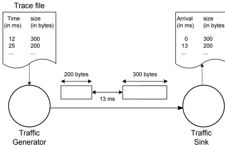
In this part of the lab, you will build a traffic generator for the trace files with Poisson traffic. In Part 3, you work with the Bellcore trace file. In Part 4, you use the VBR video traffic.
