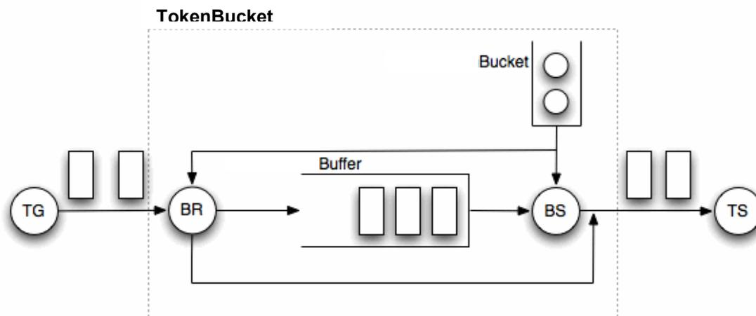
The reference implementation of the Token Bucket implements the above functions, but which is missing details on the method for updating the value of TB and for computing the time  $t^*$  for waking up the Bucket Sender. This implementation is provided by the package TokenBucket, which consists of four Java classes:
