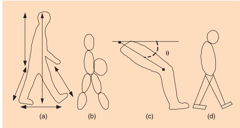
**[FIG4]** Graphical representation of parameters used in model-based approaches. (a) Distances used as static parameters in [39], (b) ellipse fitting in silhouette regions [30], (c) hip rotation model [40], and (d) model using a combination of shapes [41].
