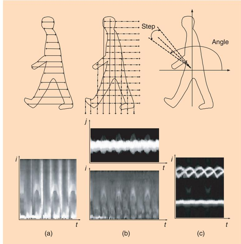
**[FIG5]** Some features extracted from binary silhouettes for gait recognition. On the bottom row, examples of these representations are shown with respect to time: (a) width of silhouette, (b) vertical (top) and horizontal (bottom) projections, and (c) angular representation.
