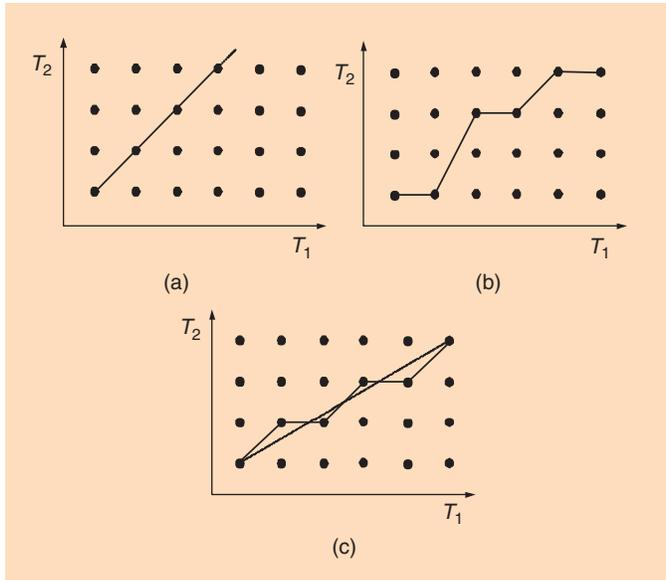
**[FIG7]** Approaches for the matching of different sequences. (a) Direct, (b) dynamic time warping, and (c) linear time normalization.
