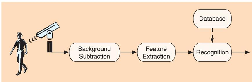
**[FIG2]** General block diagram of a gait recognition/authentication system.
