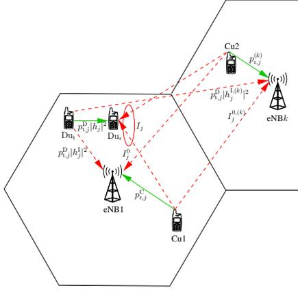
Fig. 1: A cellular network with underlay D2D users sharing uplink resources with cellular users.  $Du_t$  and  $Du_r$  denote transmit and receive nodes of a D2D pair, respectively.  $Cu1$  and  $Cu2$  denote cellular users. Solid and dashed lines denote desired and interfering signals, respectively.
