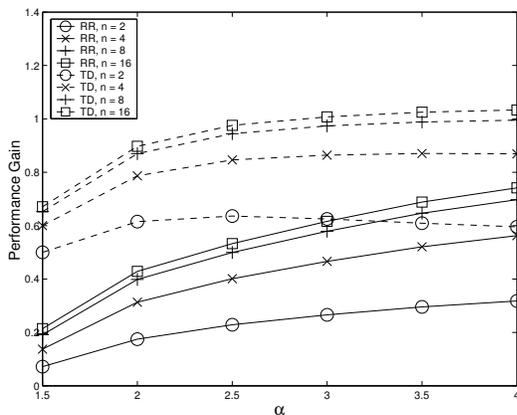
Fig. 9. Effect of roll off factor ( $\alpha$ ) and the number of relay nodes, for  $\frac{P_{ar}}{N} = 40$ ,  $\frac{P_m}{N} = 20$ ,  $\beta = 0.7$ , and  $L = 50$ .
