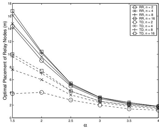
Fig. 8. Effect of roll off factor ( $\alpha$ ) and the number of relay nodes, for  $\frac{P_{ar}}{N} = 40$ ,  $\frac{P_m}{N} = 20$ ,  $\beta = 0.7$ , and  $L = 50$ .
