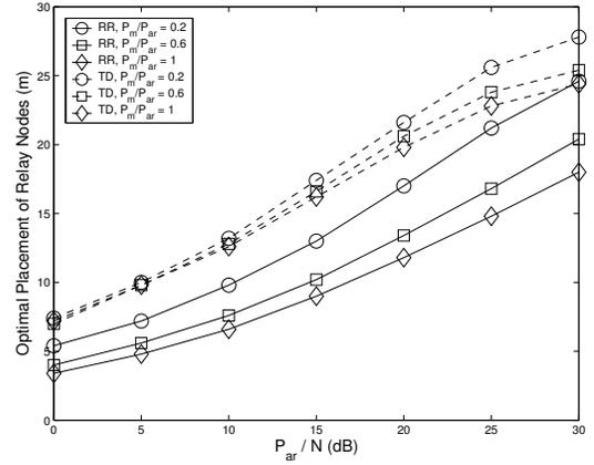
Fig. 6. Effect of the mobile to AP/RN power ratio and the AP/RN power to noise ratio, for  $\alpha = 2$ ,  $\beta = 0$ ,  $L = 50$ , and  $n = 16$ .
